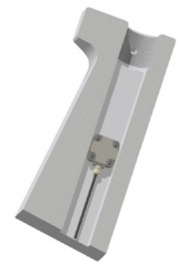
Wedge cross-section of a Hatebur press with SM type strain gauge. Fastening with M5 screws allows quick installation.
