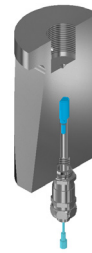
Wedge cross-section with piezoelectric strain gauge to measure the force of a given operation.
