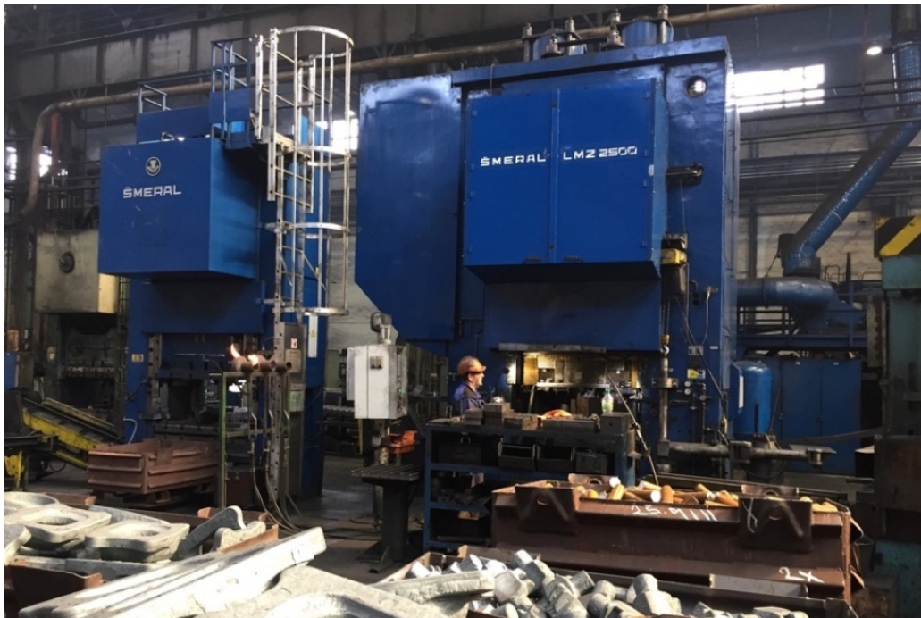
Figure 3 Different types of products are forged on the LMZ 2500 press. There are also other forging presses (hammers) nearby, which influence the vibration of the press, thus influencing the vibration analysis.
