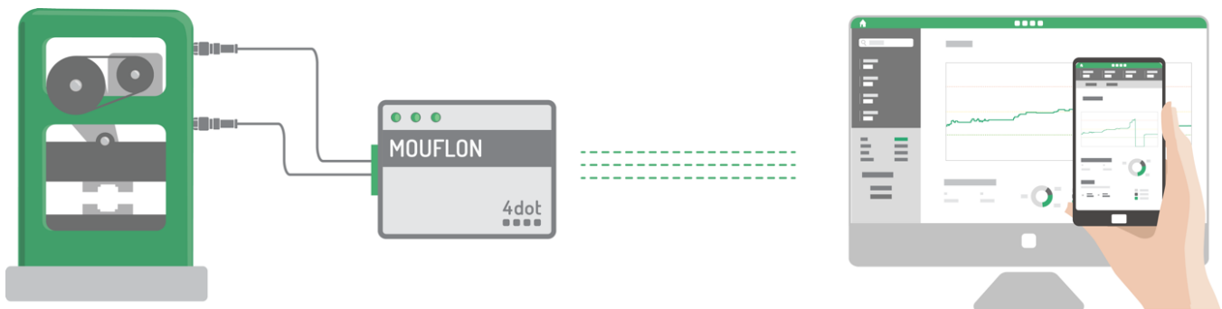
Figure 1 4dot Monitoring: the monitoring unit collects the data from sensors mounted on the machine and sends it to the cloud. The machine's condition can be monitored real-time in the 4dot application.
