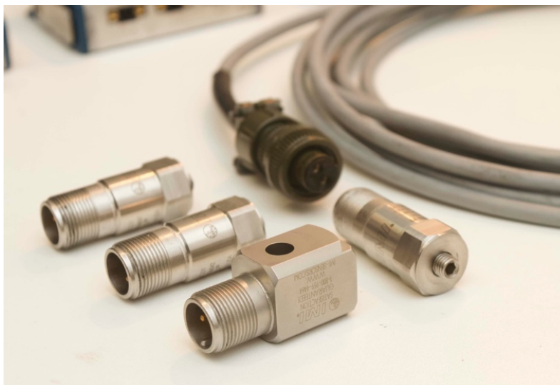
Figure 2 One-axis piezoelectric accelerometer with embedded electronics (IEPE) suitable for application on forging presses.
